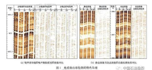
Fig.1 Special processing of electric imaging logging data for edge detection
