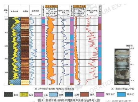
Fig.3 Comparison of evaluation results of shale macro-structure by different logging methods
